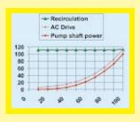
Centrifugal pumps can be controlled by methods similar to those for controlling fans. In practice, the most common method is throttling by means of a control valve. Recirculation is also used, but it is most inefficient from an energy point of view. Fitting an AC drive to the system with a 30 kW motor running 5,000 hours/year saves:
