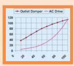
In the past, control of air flow in ventilation systems was mainly a way to alter performance, not to save energy. Although there is a number of methods, not all are energy efficient. The most basic and inefficient way of controlling the flow rate is the adjustment of a damper in the ventilation duct. Using an AC drive with a 30 kW motor running 5,000 hours/year gives the following savings:
