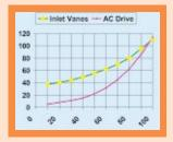
In the past, control of air flow in ventilation systems was mainly a way to alter performance, not to save energy. Although there are a number of methods, not all are energy efficient. Inlet guide vanes is a more sophisticated method for flow control, but using an AC drive instead gives the following savings for a 30 kW motor running 5,000 h per year:
