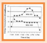
A company in New Jersey replaced the Variable Inlet Vane control (VIV) in its Air Handling Unit (AHU) with AC drive control (VSD). With 2,860 hours/year the projected savings were 61 per cent:
