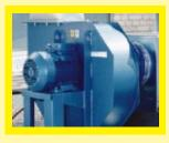
Dust is extracted from the flour milling process by 75 kW fans driven by electric motors. Fans were originally controlled by a star/delta starter, the motors running at full speed with airflow controlled by dampers. An AC drive was installed to control the fan speed.
