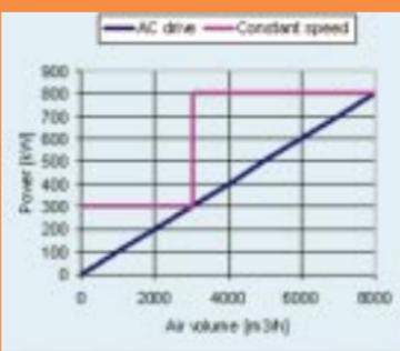
European biochemical company processes needed oxygen with constant pressure, but the oxygen volume was very variable. The system was controlled by switching on and off two compressors of different sizes. Because of problems with high power consumption, noise level and maintenance cost, the larger compressor was equipped with an AC drive. The results were:
