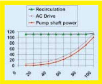
Centrifugal pumps can be controlled by methods similar to those for controlling fans. In practice, the most common method is throttling by means of a control valve. Recirculation is also used, but it is most inefficient from an energy point of view. Fitting an AC drive to the system with a 30 kW motor running 5,000 hours/year saves:
