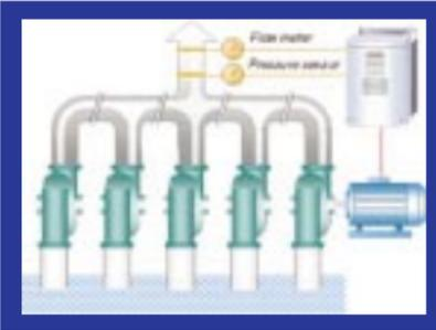
A German city waterworks improved its clean water pumping station control by installing an AC drive (185 kW). Estimated energy saving was about 50% with other benefits.
