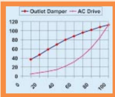
In the past, control of air flow in ventilation systems was mainly a way to alter performance, not to save energy. Although there is a number of methods, not all are energy efficient. The most basic and inefficient way of controlling the flow rate is the adjustment of a damper in the ventilation duct. Using an AC drive with a 30 kW motor running 5,000 hours/year gives the following savings:
