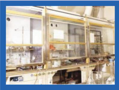
In a research laboratory, toxic materials are handled in closed glove boxes and good ventilation is required. The laboratory replaced the suction air fan's 75 kW constant speed drive with variable speed AC drive. Estimated running hours are 4,000 h/year.
