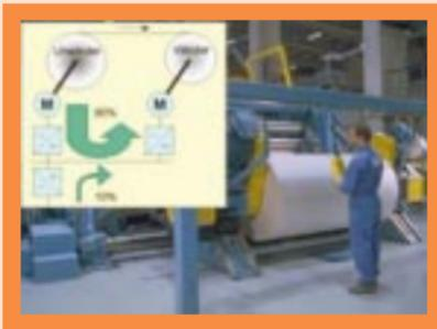
Winders and unwinders of various sizes are used in industries like paper, metal and plastics. AC drives with a common DC bus is the most efficient solution in these applications because the braking energy from unwinders can be recycled in the winder part. This example is for a 100 kW application running 8,000 hours per year.
