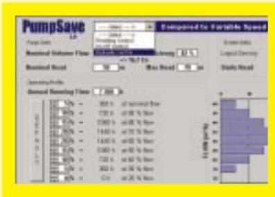
PumpSave is a calculation tool for MS Excel to estimate the energy savings available when using an adjustable frequency drive compared to other pump control systems. Calculations are based on typical pump operating characteristics. The outputs of the calculations are:
