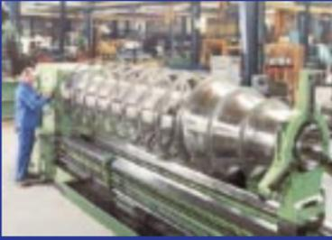
Decanters are centrifuges used to separate solid particles from liquid or slurry. A typical decanter construction is a rotating bowl with a scroll screw inside to move the solid particles out of the bowl. By using a common DC-bus solution, about half of the scroll drive power can be saved:
