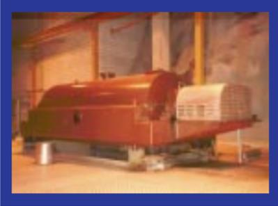
A Finnish wastewater treatment plant modernised one of its decanter centrifuges. The hydraulic system used to control the speed difference between the bowl and the scroll inside was removed and an AC drive installed instead, cutting energy consumption by 20%.
