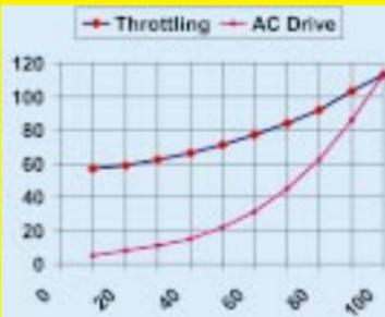
A Finnish chemical industry replaced its existing constant speed acid pump control with an AC drive (37 kW). The process is running about 8000 hours a year and the average flow is less than 50% of the pump rated flow. The results were:
