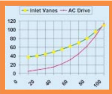
In the past, control of air flow in ventilation systems was mainly a way to alter performance, not to save energy. Although there are a number of methods, not all are energy efficient. Inlet guide vanes is a more sophisticated method for flow control, but using an AC drive instead gives the following savings for a 30 kW motor running 5,000 h per year:
