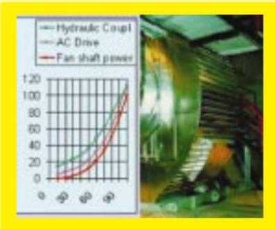
A Finnish pulp mill compared hydraulic coupling to AC drive (1,370 kW) for its power plant ID (Induced Draft) fan. The power plant is running continuously and the flue gas flow varies from 50% to 90% of the maximum capacity. With AC drive:
