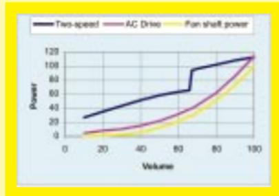
A quite simple way of controlling the flow rate is the use of a two-speed motor, but it has two flow rates only. Using an AC drive instead gives the following savings for 30 kW motor running 5,000 h per year:
